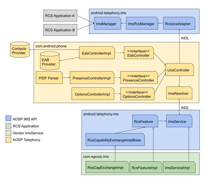
**Figure 3.5.1**: High level summary of the changes required to support UCE in AOSP. The RCS applications will use the ImsManager API to request the cached capabilities of contacts or request availability queries from the network. AOSP Telephony will control UCE and send requests to the vendor ImsService when necessary to publish capabilities and subscribe to the capabilities of one or more contacts.
