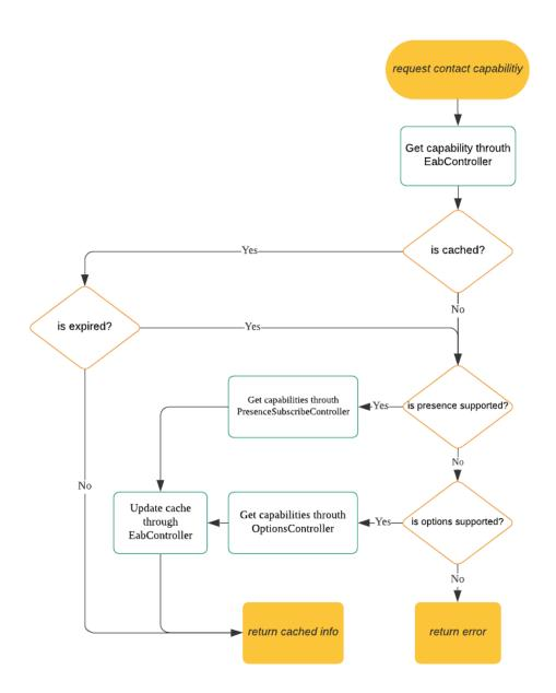
Figure 3.5.3: Flow diagram showing the caching behavior of AOSP for real-time availability (top) and capability requests (bottom) of a contact.
