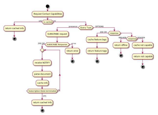
Figure 3.5.2: Flow diagram showing the caching behavior of AOSP for the RCS capabilities of the user's contacts.
