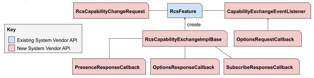
Figure 3.5.6: The modified system API surface used for UCE as part of the ImsService API.
