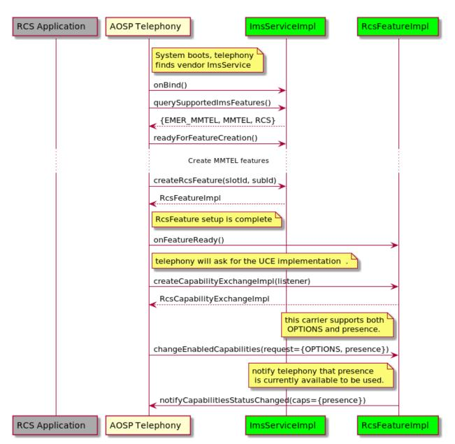
**Figure 3.5.7:** The typical setup flow of the RcsFeature associated with the ImsService and creation of the vendor RcsCapabilityExchangeImplBase implementation.
