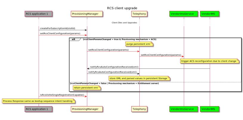
Scenario P.EC.5: Reconfiguration triggered by the RCS application due to 403 forbidden
